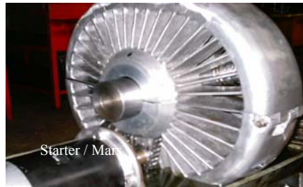
Figure 4.1. First installation of the elliptic engine (closed body) Şekil 4.1. Eliptik motorun ilk montajı (gövde kapalı)
