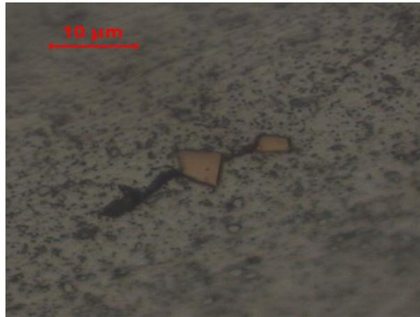
Figure 10. Image of crack initiation in valve table.
