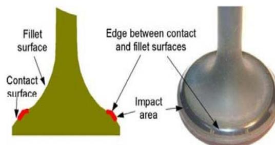
Figure 2. Location of impact area on the exhaust valve.
