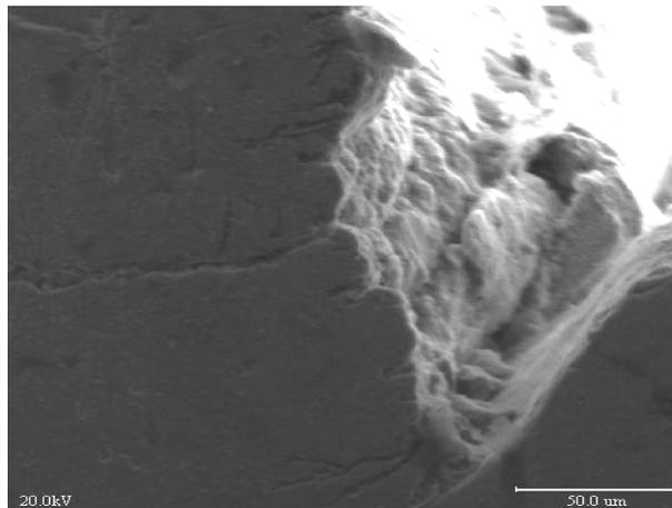
Figure 4. SEM image of the fracture surfaces of the failed valve.
