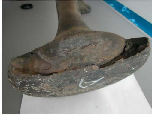
Figure 3. Catastrophic failure on the valve table.
