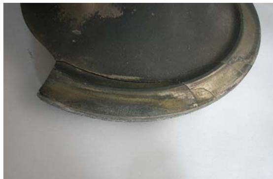
Figure 1. Cracks on table of failed exhaust valve.
