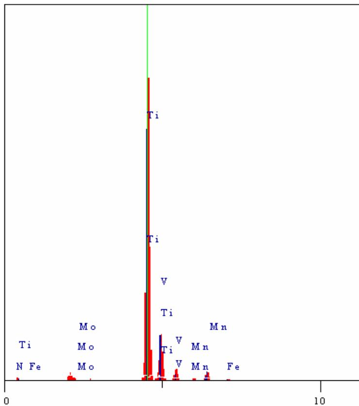
Figure 9. EDS analyse results of the point shown in Figure 8.
