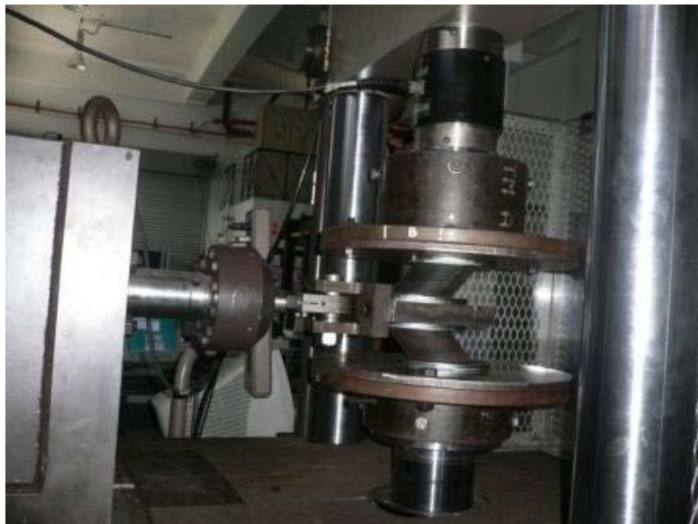
Figure 6. Double Shear Testing Setup of Rubber Bearing by ETM.
