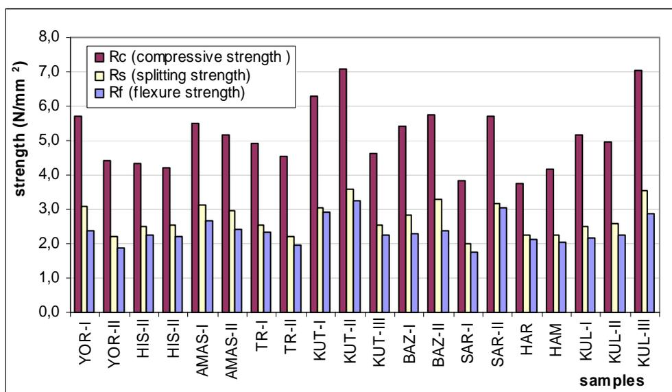
Figure 3. Mechanical properties of the lime mortars produced of powder brick
