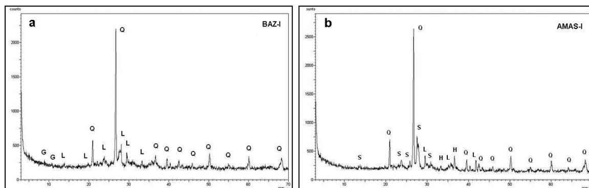
Figure 9. X-ray diffractions of (a) Roman Basilica brick and (b) Roman Amasra Castle brick (AMAS-I). (*Q*: Quartz, *L*: labradorite, *H*: hematite *G*: Glaucofanane, *S*: Sanidine,
