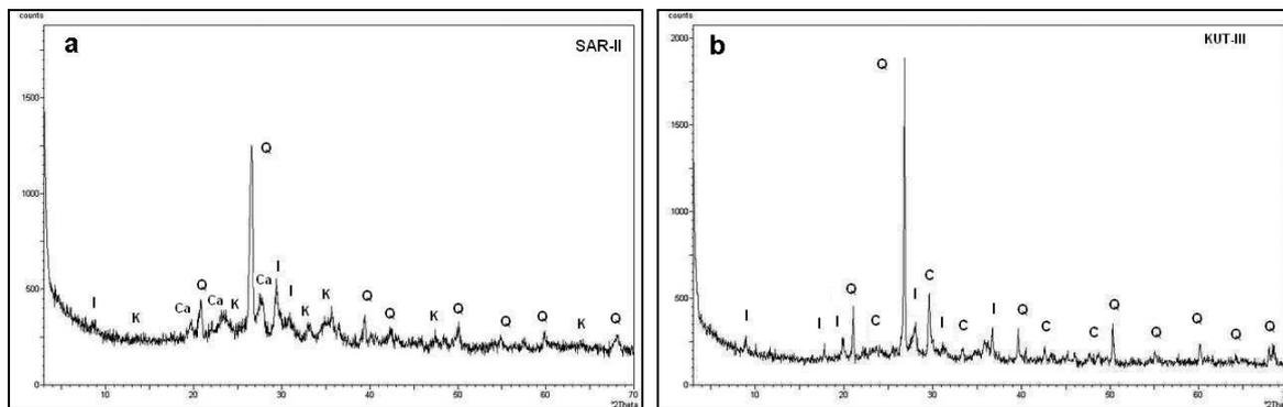
Figure 5. X-ray diffractions of (a) Ottoman Cistern (SAR) and (b) Kütahya Castle (KUT-III) bricks (*Q*: Quartz, *Ca*: Calcium oxide, *I*: Illite, *K*: Cyanite, *C*: Calcite)
