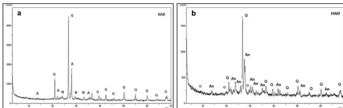
Figure 8. X-ray diffractions of (a) Mill brick (HAR) and (b) Ottoman Bath brick (HAM) (*Q*: Quartz, *A*: albite, *An*: anorthoclase, *L*: labradorite, *H*: hematite, *G*: Glaucofanane, *O*: Orthoferrosillite)
