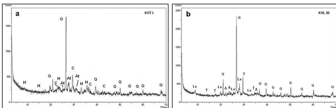
Figure 6. X-ray diffractions of (a) Kütahya Castle (KUT-I) and (b) Yedikule City Wall (KUL-III) bricks (*Q*: Quartz, *At*: Anortite, *A*: albite, *C*: Calcite, *H*: hematite, *Le*: Lepidolite, *T*: Tourmaline)
