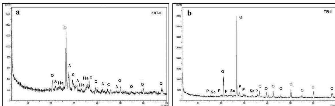
Figure 7. X-ray diffractions of (a) Kütahya Castle (KUT-II) and (b) Trabzon Castle (TR-II) bricks (*Q*: Quartz, *A*: albite, *Ha*: Halloysite, *C*: Calcite, *P*: Pyroxene, *So*: Sodium silicate)
