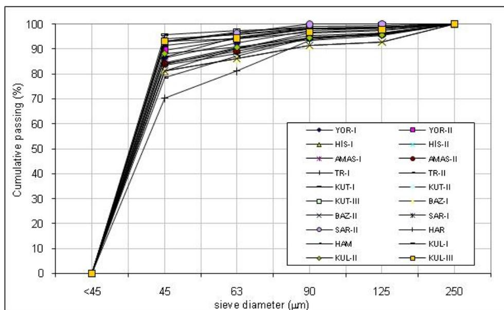
Figure 2. Granulometric distribution of ground brick samples
