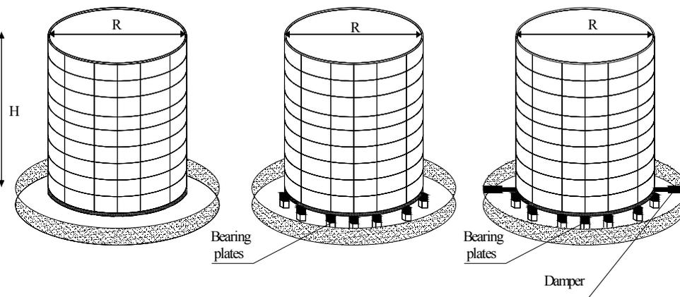
Figure 3. Reference and seismic isolated liquid storage tank models
