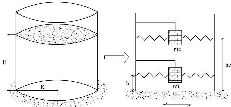
Figure 2. Equivalent of full of liquid storage tank as modeled single freedom degree.
