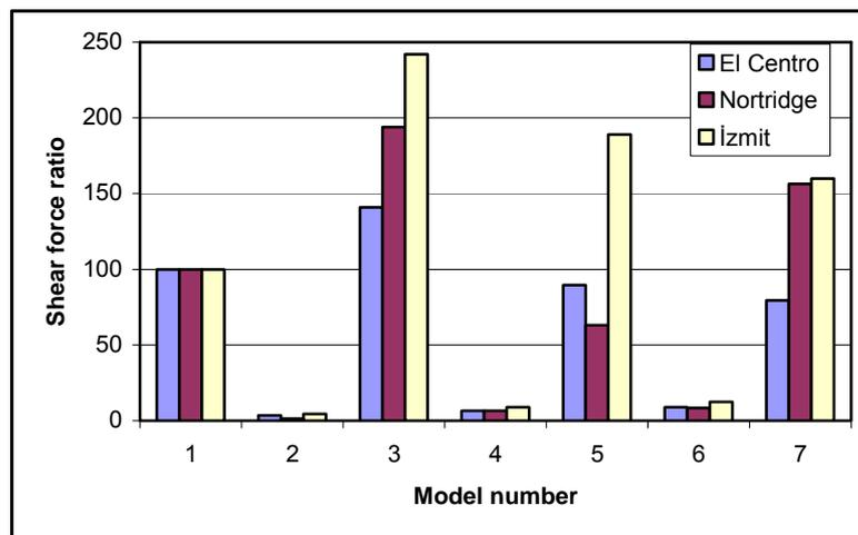
Figure 4. Ratio of shearing force occurred at base of tank models
