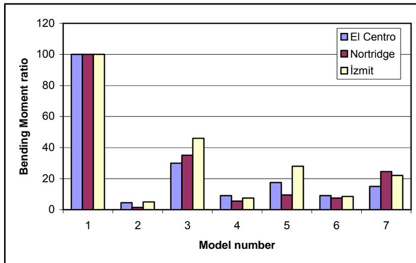
Figure 5. Ratio of moment occurred at base of tank models
