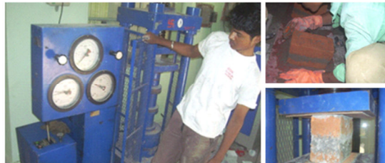
Fig. 6. Brick mortar joint crushing strength test set-up
