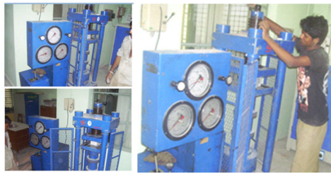
Figure 5. Cement mortar compressive strength test set-up
