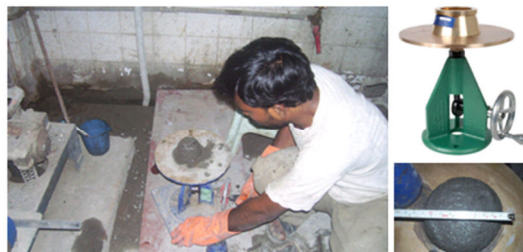
Figure 4. Flow table test set-up
