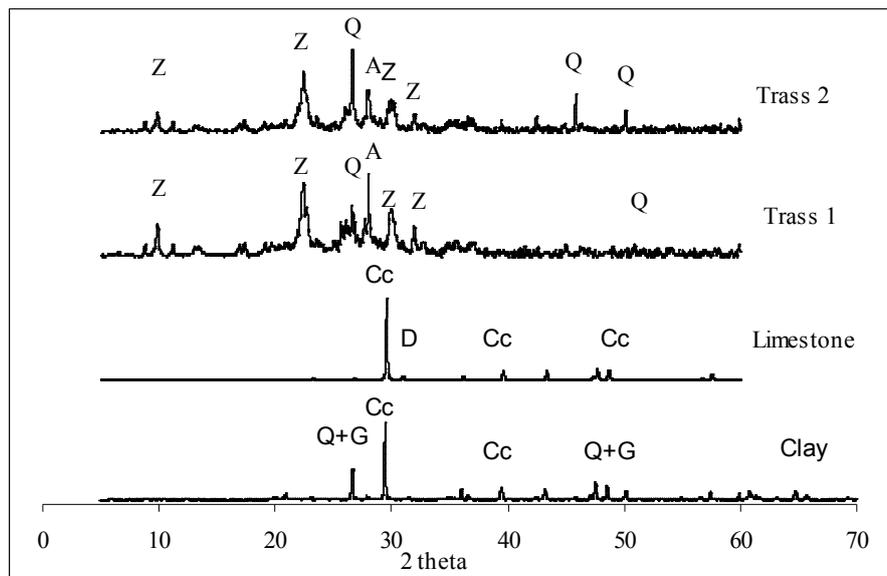
Figure 1. XRD analysis of the raw materials limestone, clay, trass 1 and trass 2.
