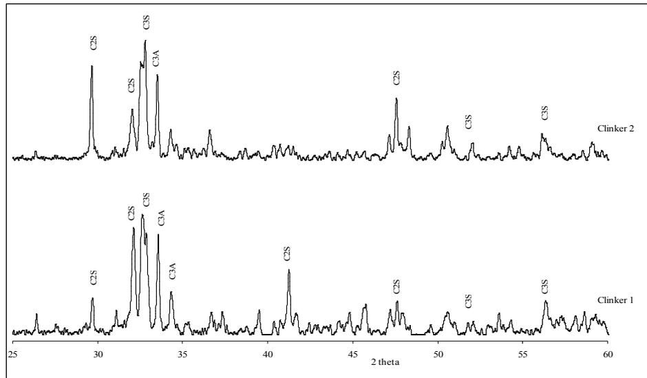
Figure 3. The XRD analysis of clinker 1 and clinker 2.
