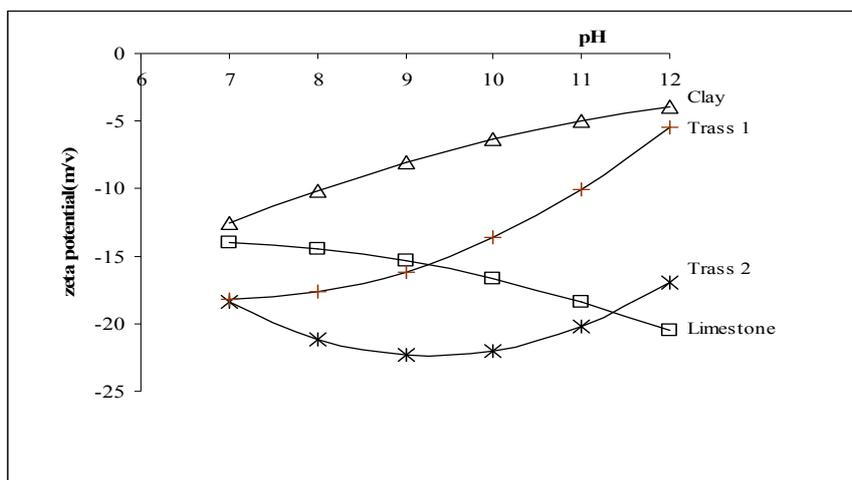
Figure 2. The change of the zeta potential depending on the pH value of limestone, clay and trasses 1 and 2.
