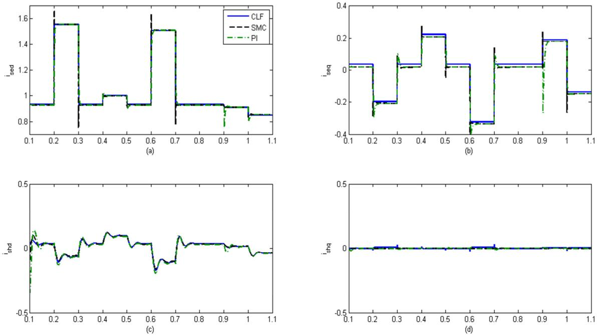
Fig. 4. Response of the UPFC system with 10% uncertainty. solid line: proposed CLF, dashed line: proposed SMC, dash-dot line: PI controller with no uncertainty.
