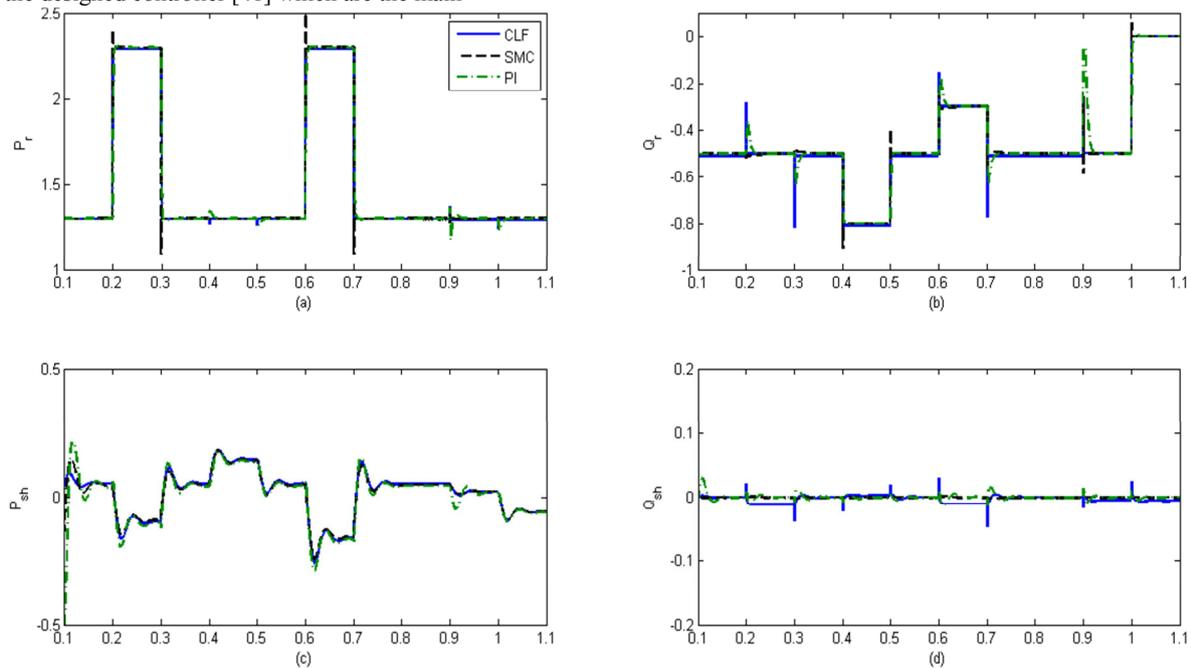
Fig. 3. Response of the UPFC system with 10% uncertainty according to the case studies. solid line: proposed CLF, dashed line: proposed SMC, dash-dot line: PI controller with no uncertainty. (a) active power of the transmission line, (b) reactive power of transmission line, (c) active power of the shunt converter, (d) reactive power of shunt converter.
