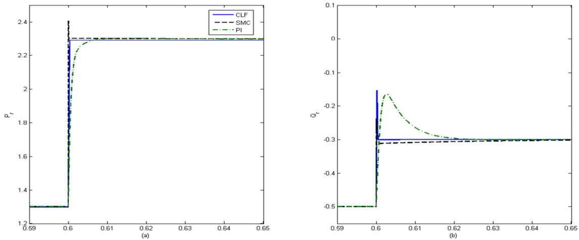
Fig. 6. Scaled response of the UPFC system with 10% uncertainty at  $t=0.6$ . solid line: proposed CLF, dashed line: proposed SMC, dash-dot line: PI controller with no uncertainty.
