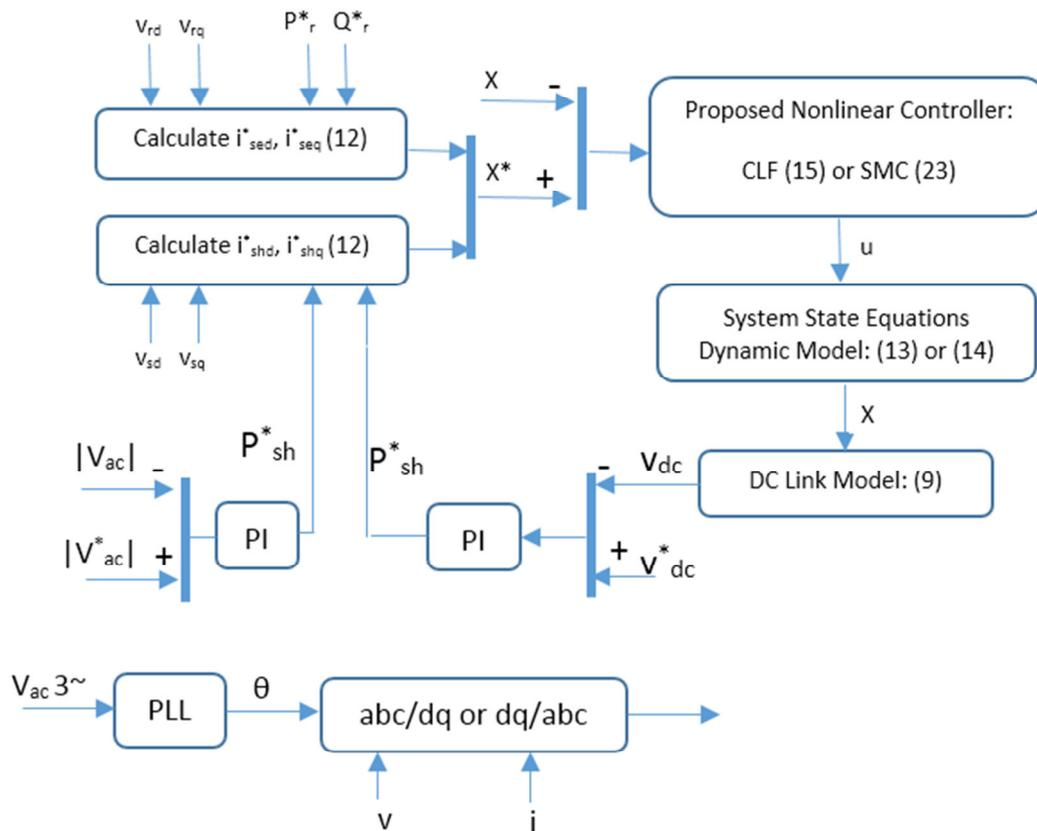
Fig. 2. Schematic diagram of the proposed nonlinear controllers
