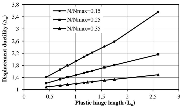
**Figure 4.** Plastic hinge length-displacement ductility curve for different axial load
