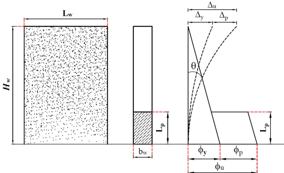
**Figure 1.** Theoretical model of cantilever shear walls.
