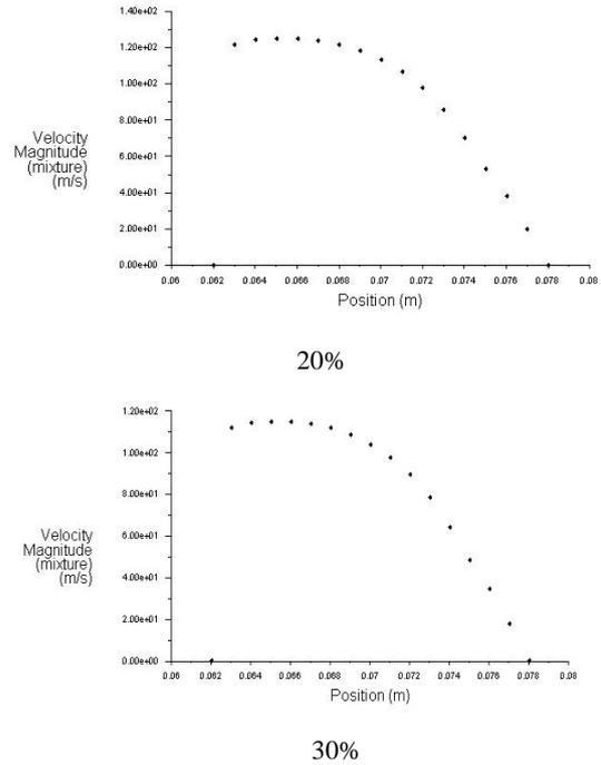
Fig.3 Outlet velocity of abrasive with different volume fraction
