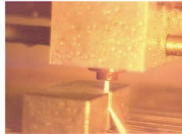
Fig.6 45 # steel cutting
