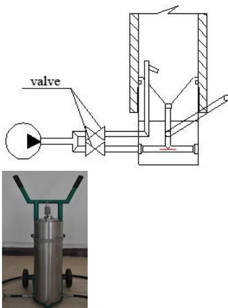
Fig.5 Assembly drawing of abrasive mixing chamber
