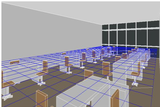
Figure 1. Sample Office, sensor placement on 75 cm height and light shelf on facade.
