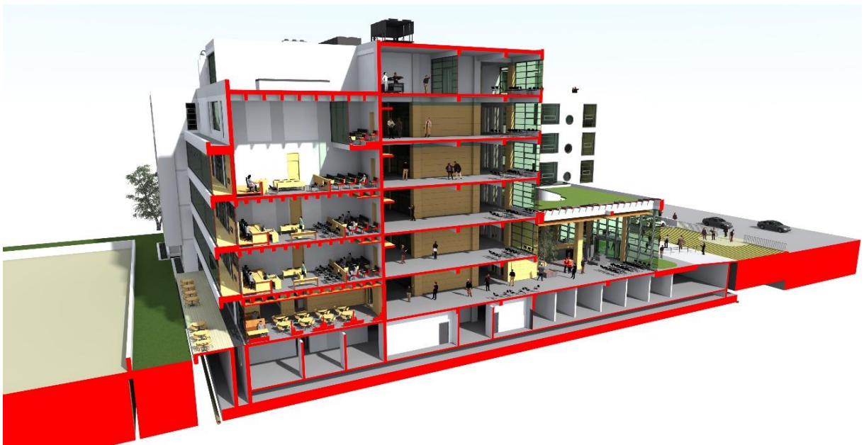
Figure 6: Section of the Building – Relationship Between Judge Corridor and Public Circulation is Showed
