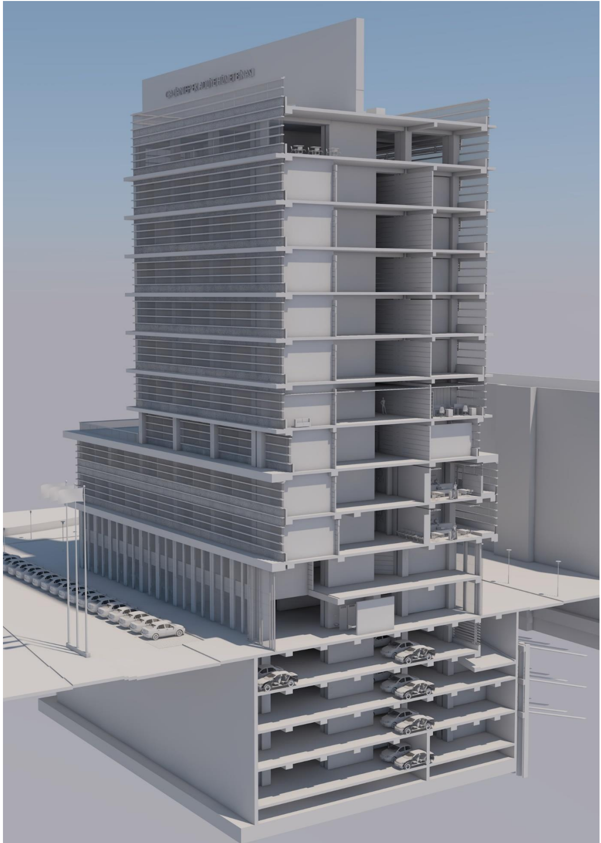
Figure 8: Section Perspective of Gaziantep Annex Courthouse Building
