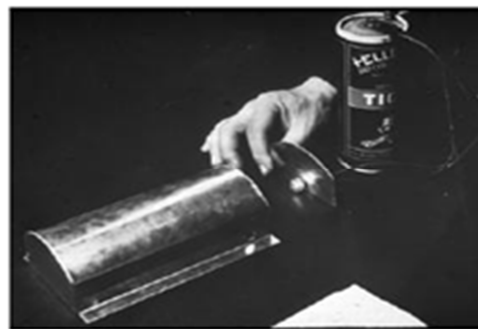
Figure 9. Optical model of a hall with a concave ceiling. The energy distribution on the floor can be studied on a photographic plate [5].
