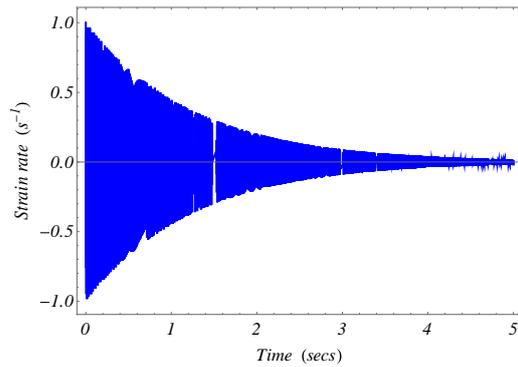
Case 1: Vibration Damping Impulse Response at  $x_0 = 2.3$  cm
