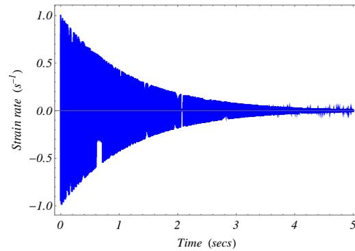
Case 2: Vibration Damping Impulse Response at  $x_0 = 3.3$  cm
