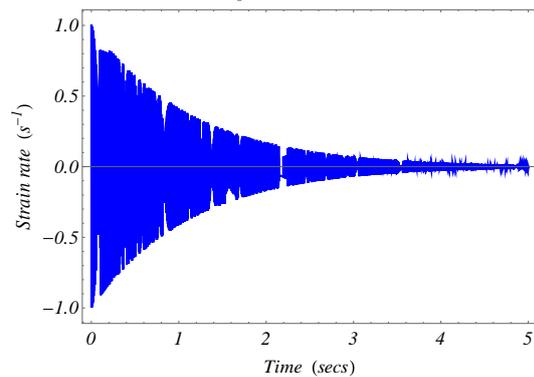
Case 4: Vibration Damping Impulse Response at  $x_0 = 5.3$  cm
