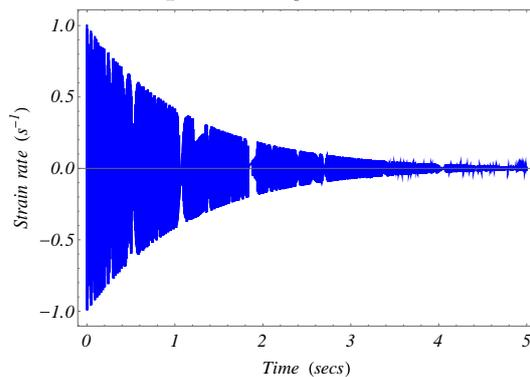
Case 3: Vibration Damping Impulse Response at  $x_0 = 4.3$  cm
