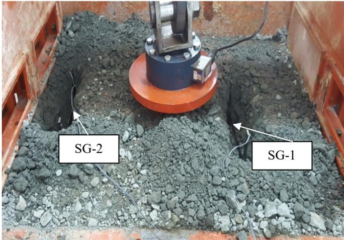
*Figure 3 - Strain gauge placements in the base layer*
