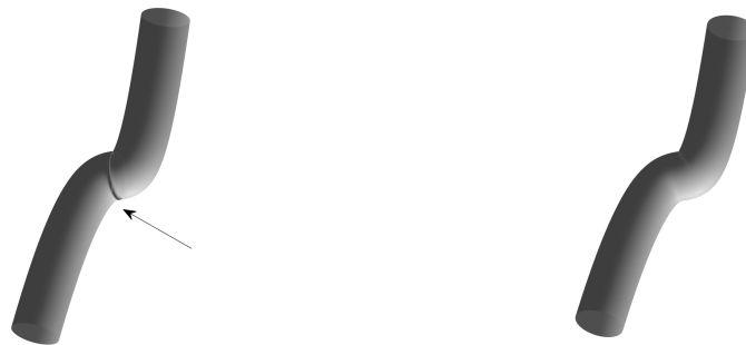
Figure 9. The tube surfaces generated by Frenet frame (left) and the Flc-frame (right) t \in (-2, 2), v \in (-4, 4) .
