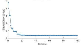
Fig. 11 - Convergence history for the Cantilever beam design problem
