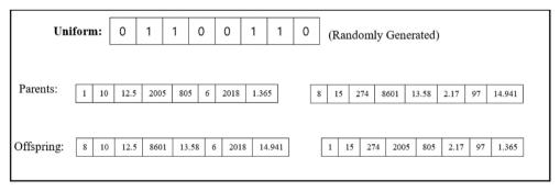
Fig. 4 - Schematic of Uniform crossover
