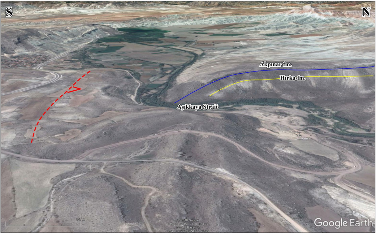
Figure 7- a) Inclined Google Earth image of the asymmetric anticline formed by the layers of the Akınar and Hırka formations in the Aşikkaya strait. The probable position of the Uzunbayır Blind Thrust in front of the 30° dipping limb is indicated by a dashed red line. The thrust planes can be traced on the surface at eastern and western edges of the study area. See figures 7b and c.
