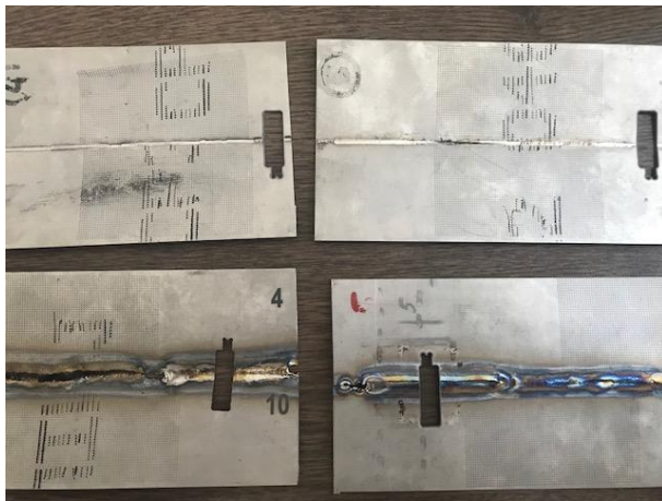
Figure 2. The welded specimens a) Pulsed fiber laser welding specimen (L1) b) Pulsed fiber laser welding specimen (L2) c) TIG welding specimen (T1) d) TIG welding specimen (T2).
