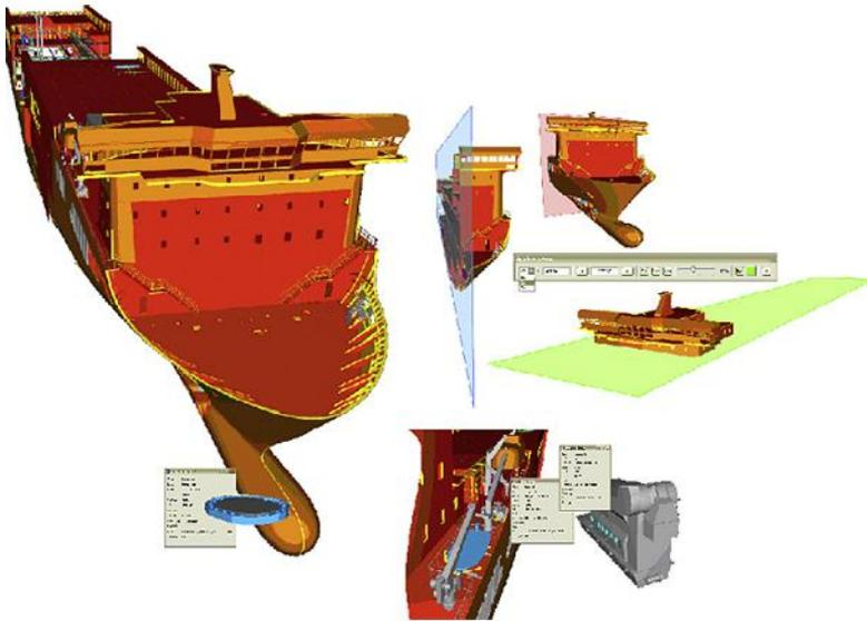
**Figure 1.** The interior view of a ship with clip plane (Source: [4]).
