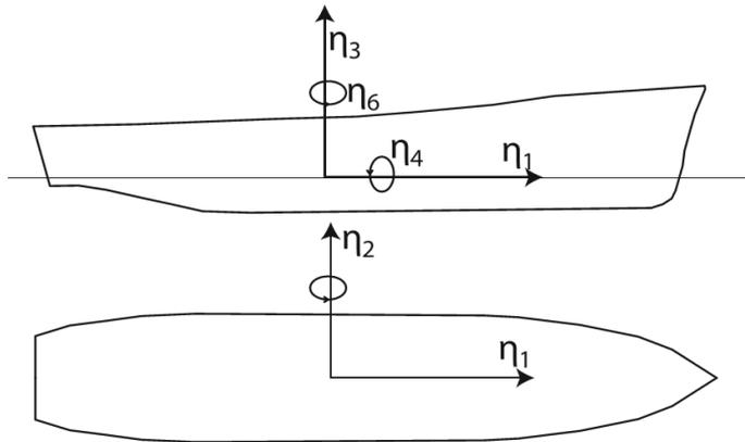
**Figure 3.** Ship coordinate system (Source: [5]).
