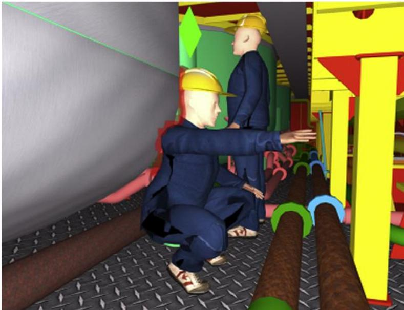
**Figure 2.** Ergonomic check of the design using dummies (Source: [1]).
