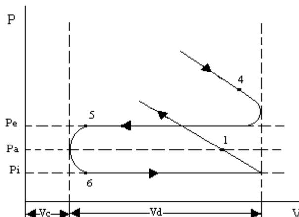
**Figure 4.** Gas Exchange Processes in the Engine Cylinder.
