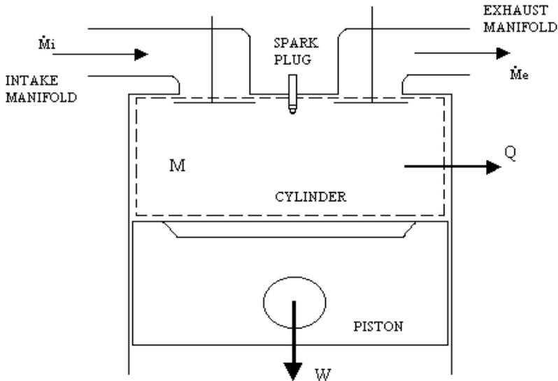
Figure 3. Engine Cylinder Thermodynamic System.
