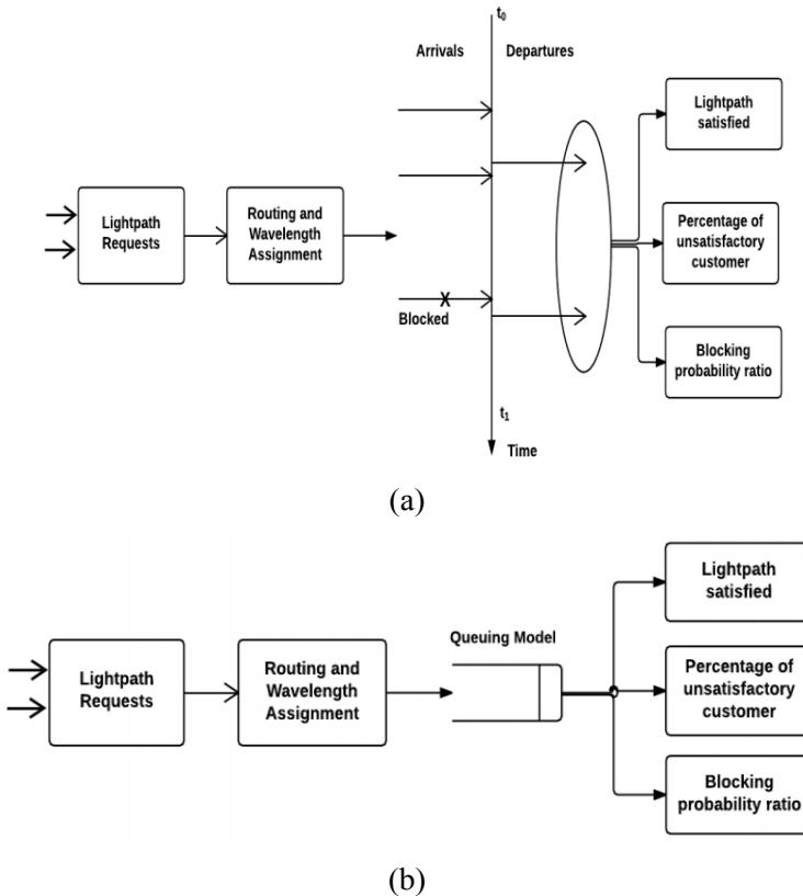
**Figure 2.** (a) Proposed scheme without queuing approach (b) Proposed scheme with queuing model (with SDN paradigm).
