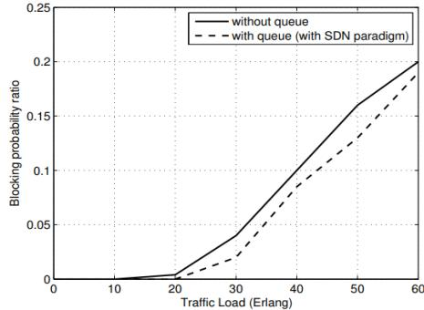
**Figure 6.** Blocking probability ratio w.r.t traffic load.
