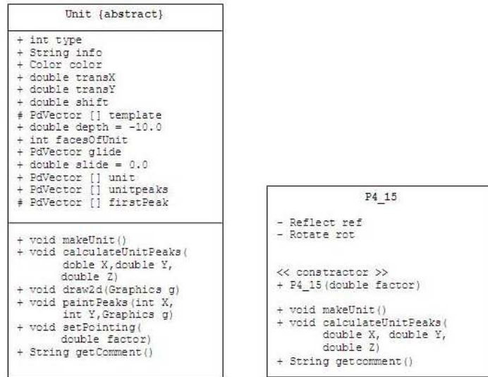
Figure 4. The UML diagram of the Unit abstract class and the p4_15 parameter class
