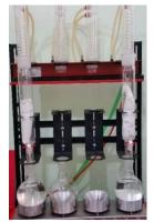
Figure 4. Soxhlet used for oil extraction
