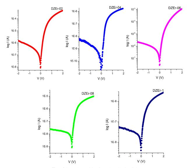
Figure 3. logI-V characteristics of DZEr heterojunction diodes
