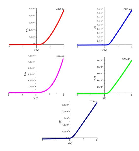
Figure 2. I-V characteristics of DZEr heterojunction diodes
