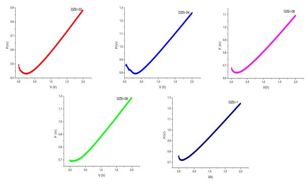
Figure 4. F(V)-V plots of DZEr heterojunction diodes
