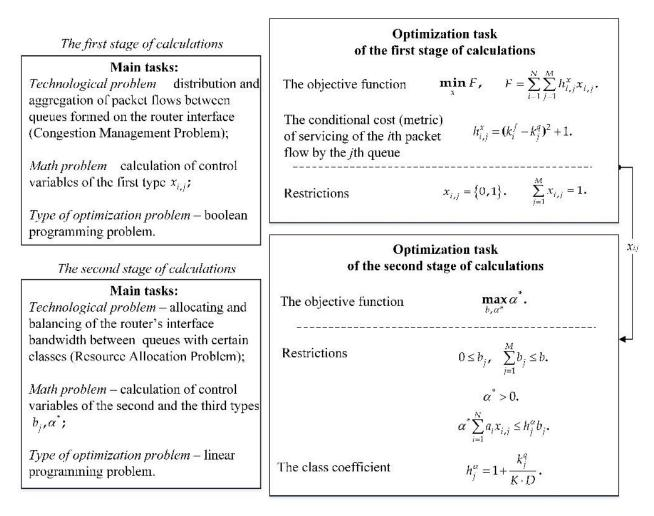
Figure 1. The structure of the method of congestion management and balanced resource allocation on MPLS-TE telecommunication network routers.
