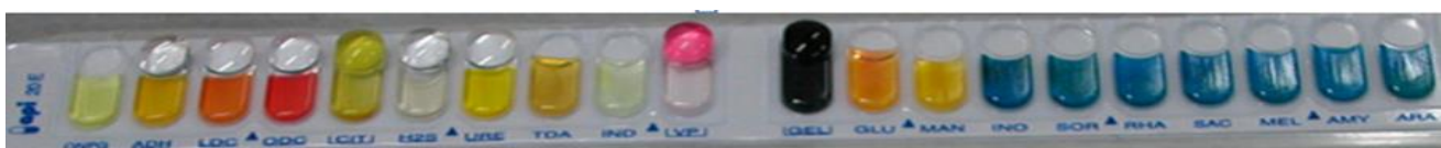
Figure 3. Biochemical test results of Y. ruckeri strain with API 20 E test kit (Original).
