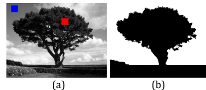
Figure 6. (a) Second group seed sample (b) SRG segmentation result of the second group seed sample
