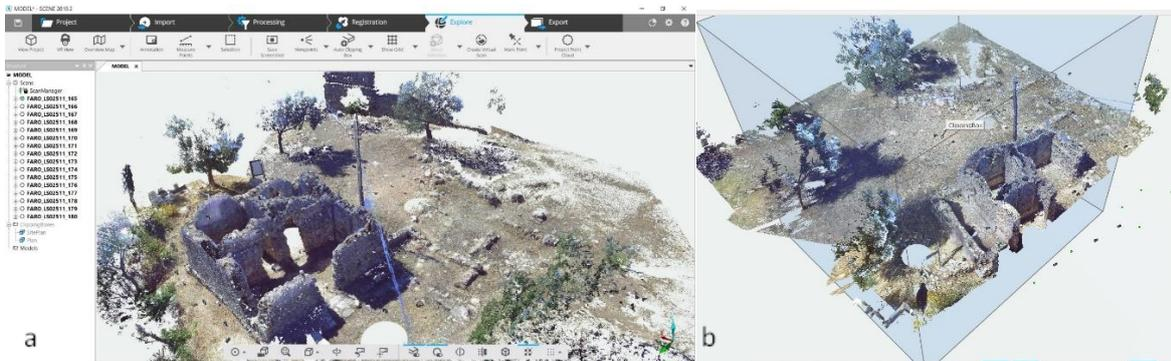
Fig.5 The program interface and the point cloud of the bath (a) and clipbox command (b)
