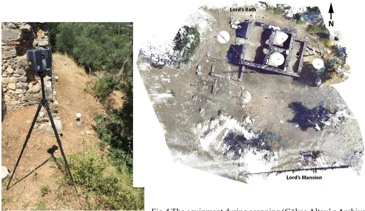
Fig.4 The equipment during scanning (Gökçe Altay' s Archive, 2019) (a) and scanned area (b)
