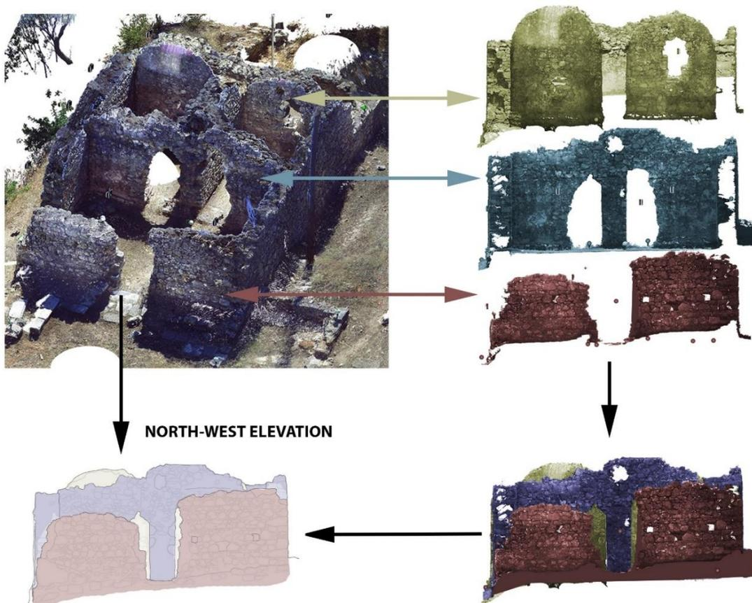
Fig.6 Diagram showing production of a facade drawing
