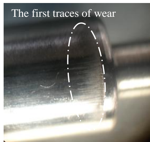
Figure 4.7. Photo injector needle at the end of 400 hours of work
