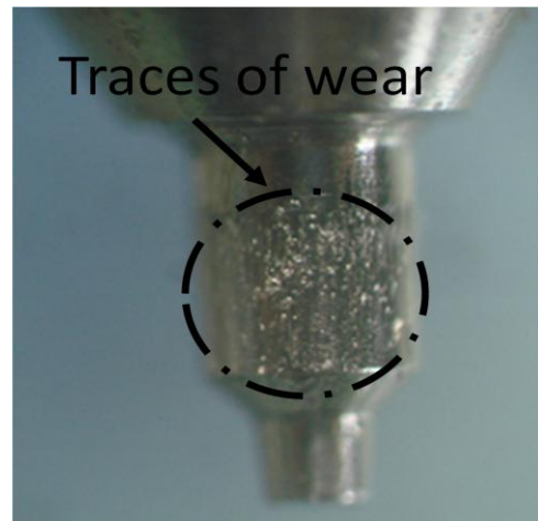
Figure 4.9. Photo injector needle at the end of 1000 hours of operation
