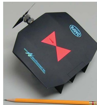
Figure 5. Black Widow Fixed Wing MAV [13]
