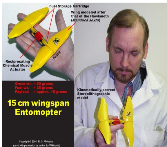
Figure 7. Entomopter for Mars Exploration Mission [18]
