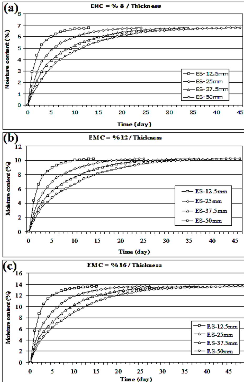
Figure 3. Moisture content change of the samples according to different thicknesses in adsorption case for EMC = 8% (a), 12% (b) and 16% (c)
