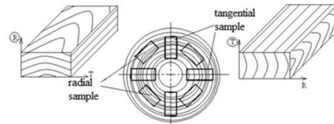
Figure 1. The cross sections of radial and tangential samples
