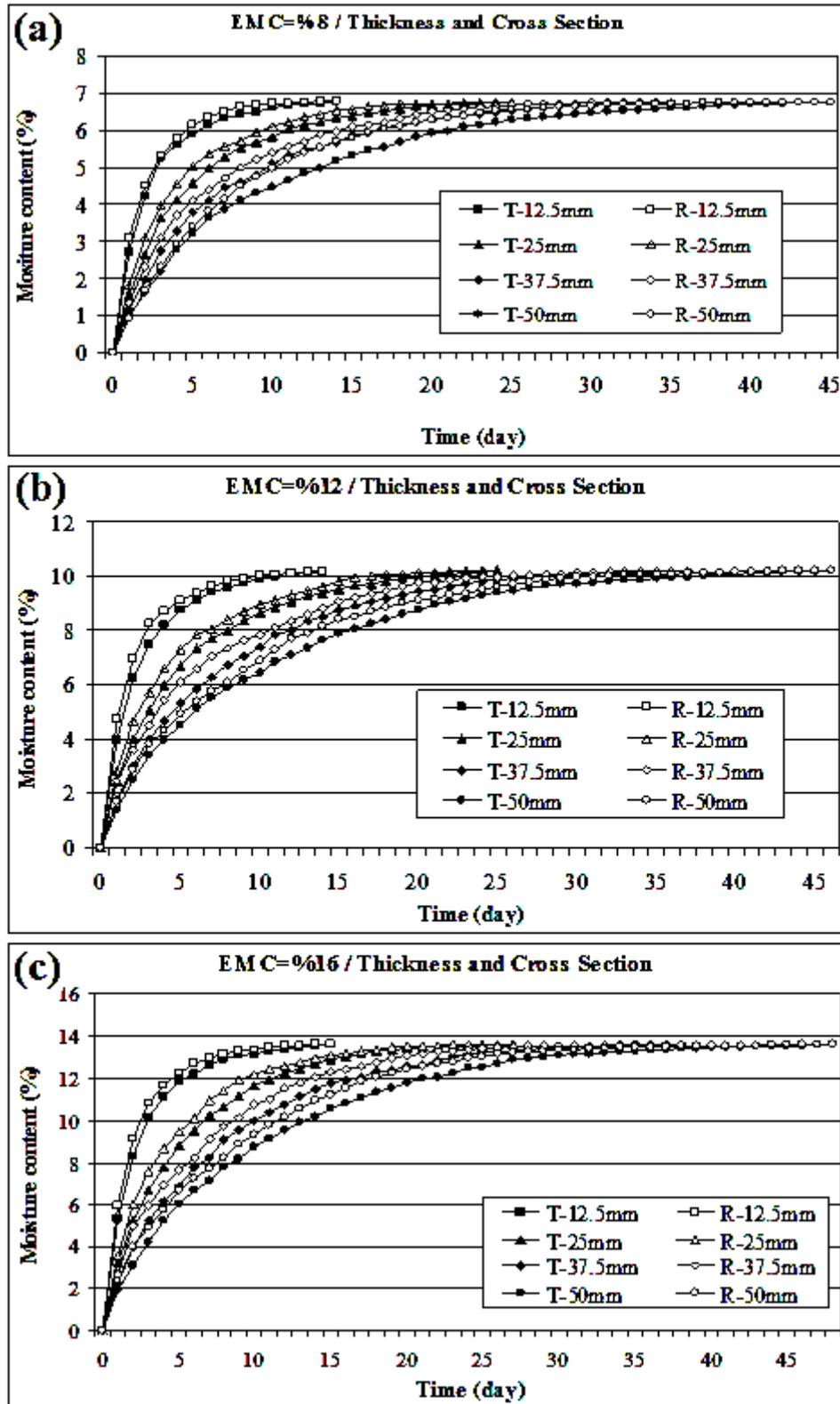
Figure 2. Moisture content change of the samples according to their section and width in adsorption case for EMC = 8% (a), 12% (b) and 16% (c)
