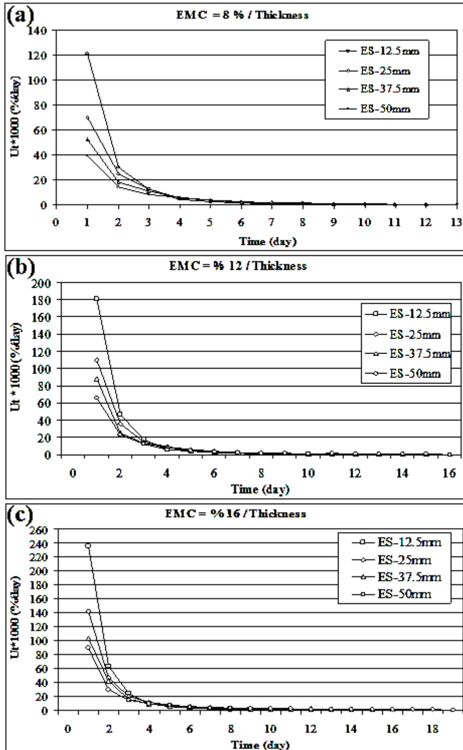
Figure 4. Wood adsorption speed for EMC = 8% (a), 12% (b) and 16% (c)
