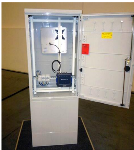
Figure 5. Inside of reader RFID gate [4]
