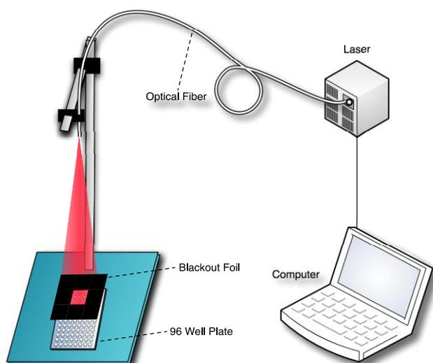
**Figure 1.** Laser set-up for experiments.
