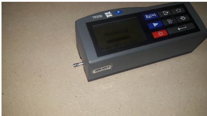
Figure 1: Measurement of surface roughness parameters of MDF by stylus contact tester
