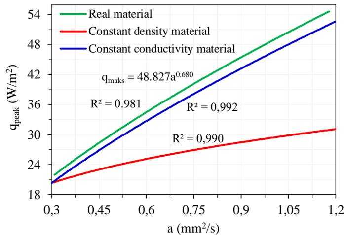
**Figure 11.** Comparison of the effect of the thermal diffusivity on the peak heat gains through the walls for real material and constant property material.
