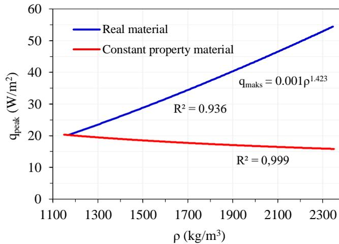
**Figure 6.** Comparison of the effect of the density on the peak heat gains through the walls for real material and constant property material walls due to south direction.
