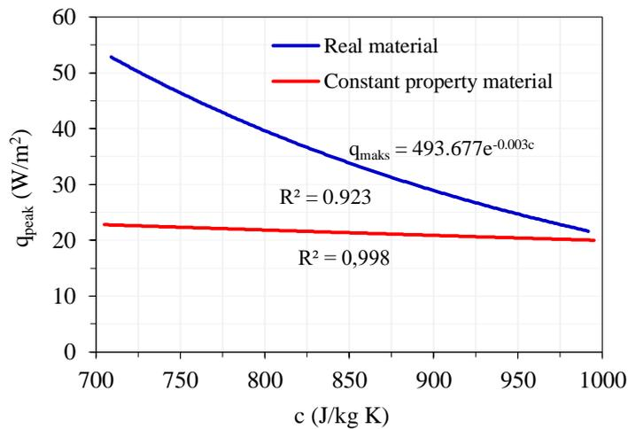
**Figure 8.** Comparison of the effect of the specific heat on the peak heat gains through the walls for real material and constant property material.
