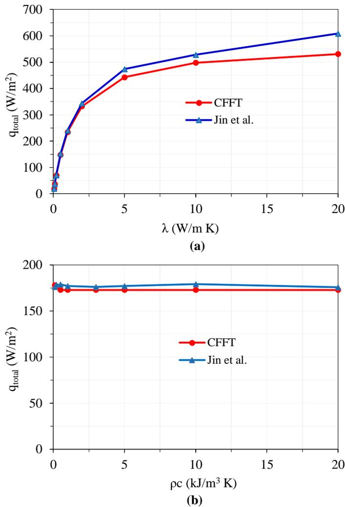
**Figure 1.** A comparison between the method of Jin et al. [16] and CFFT in the calculation of heat flux due to the variation of thermophysical properties: (a) with constant heat capacity (b) with constant thermal conductivity
