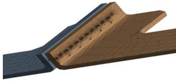
Figure 7. The mesh of the unidirectional model
