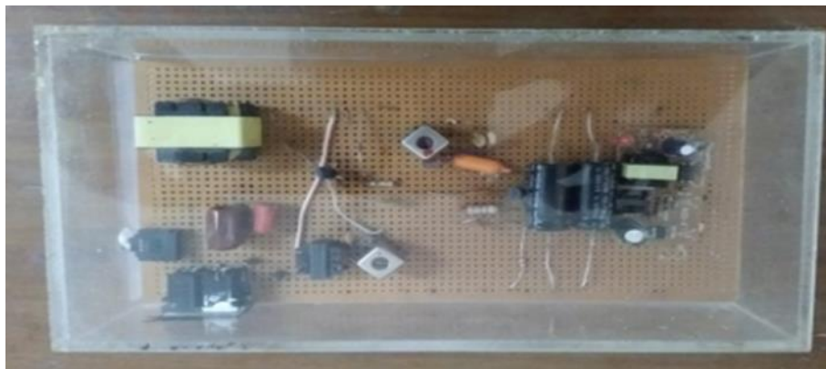
Fig 6. Modem at transmission side consisting of power supply, Oscillator, modulator and coupling circuit.
