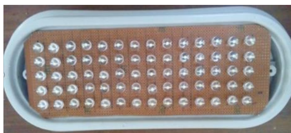
Fig 9. LED panel consisting of 72 LEDs, (14 x 5).
