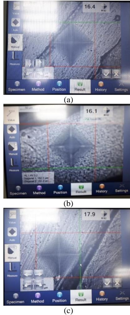
**Figure 8.** Micro hardness measurements (a) 25% with diamond infill, (b) 15% with diamond infill, (c) 75 % with linear infill.
