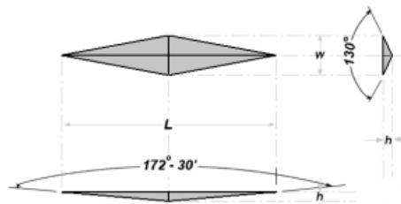
**Figure 5.** The Knoop Hardness Indentation [13].
