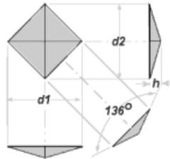
Figure 6. Vickers Pyramid Diamond Intender [13].
