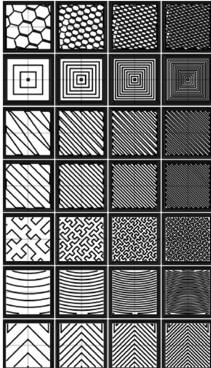
**Figure 1.** Infill types at different densities (Left to Right: 20%, 40%, 60% and 80%. Top to Bottom: Honeycomb Concentric, Line, Rectilinear, Hilbert Curve, Archimedean Chords, Octagram Spiral) [6].
