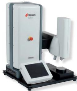
Figure 7. EMCO-TEST DuraScan micro hardness test machine.
