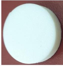
**Figure 4.** The produced disc shape specimen for hardness measurement.
