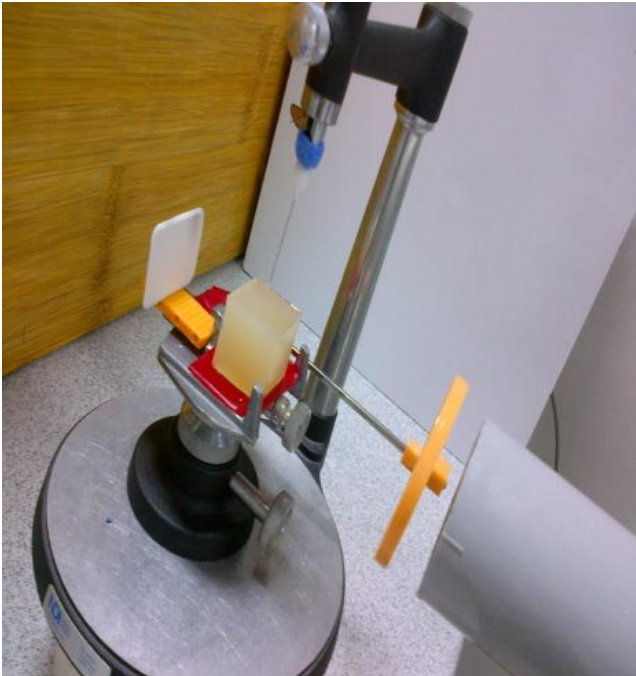
Figure 7. Standard mold mounted on surveyor with cone parallel device used.
