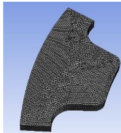
Fig. 4. 1/12 cyclic symmetry finite element model
