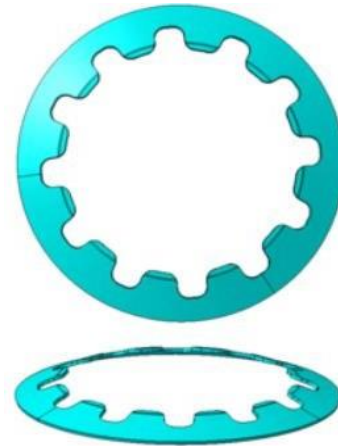
Fig. 3. Belleville spring solid geometry
