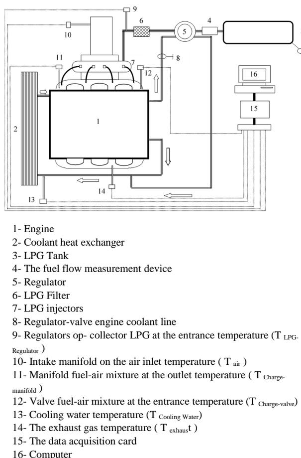
Figure 2 Detailed schematics for LPG flow line and engine coolant circuit
