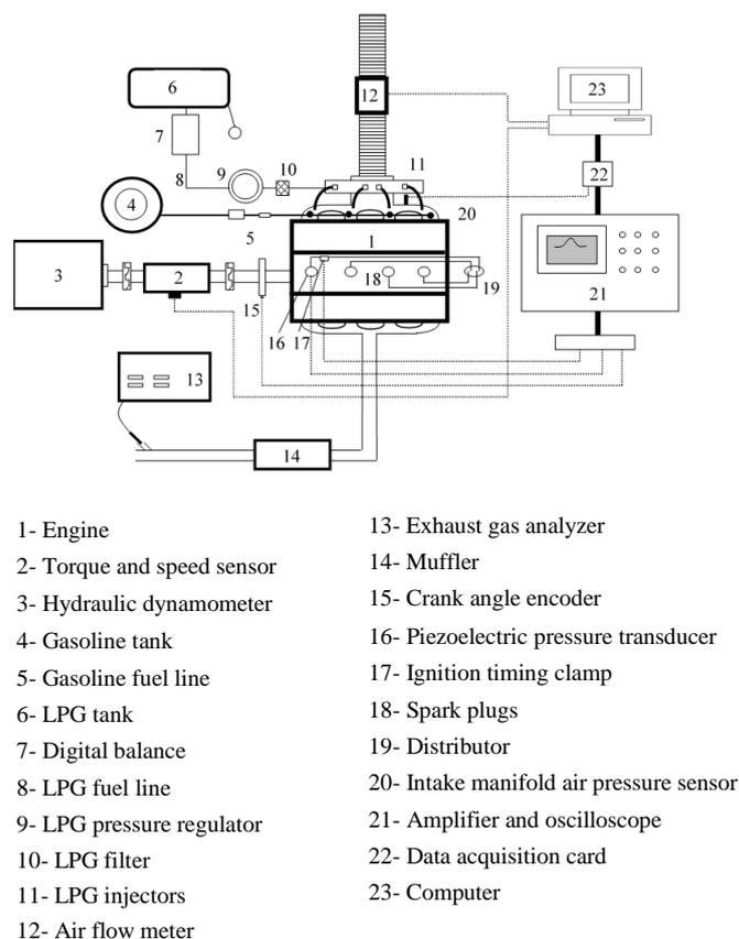
Figure 1. A schematic view of the test set-up
