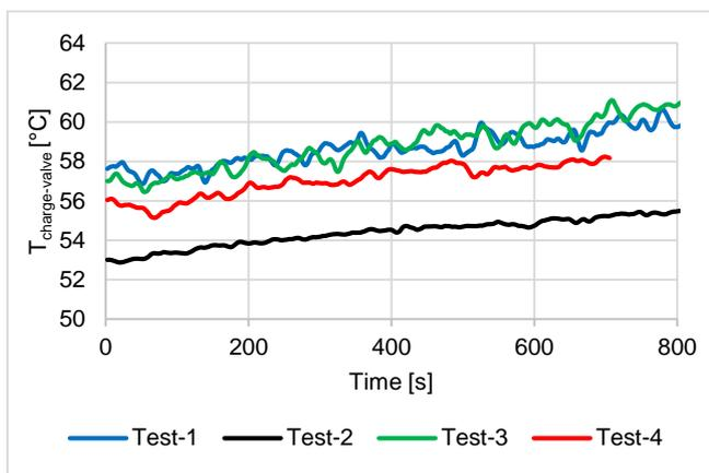
Figure 5. Temperature of fuel-air mixture at entrance of valve ( $T_{\text{charge-valve}}$ )
