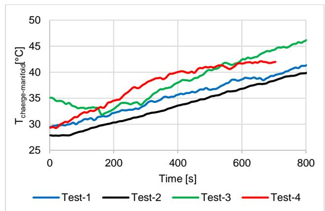
Figure 4. Temperature of fuel-air mixture at manifold output ( $T_{charge-manifold}$ )
