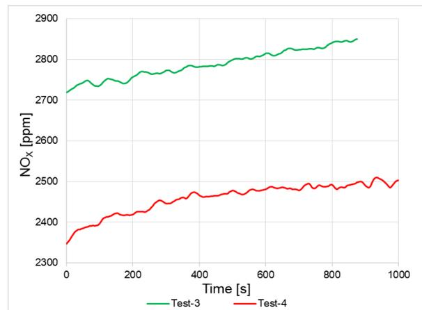
Figure 11. Variation of NOx emission with time for Test-3 and Test-4
