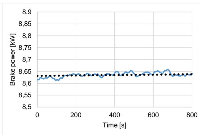
Figure 6. The variation of effective power with time for Test-1
