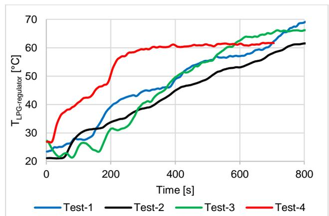
Figure 3. LPG temperature at regulator outlet ( $T_{LPG-regulator}$ )
