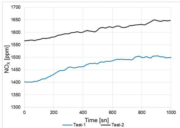
Figure 10. Variation of NOx emission with time for Test-1 and Test-2
