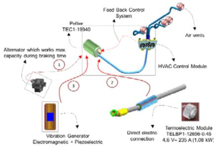
Figure 10. Varying electricity generators used in the developed system
