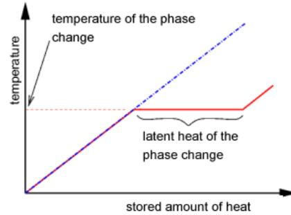
**Figure 8.** Storing heat at steady temperature [10]
