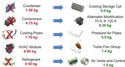
Figure 11. Current and developed system components and weigh
