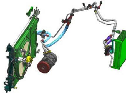
**Figure 2.** Current air conditioning cooling group
