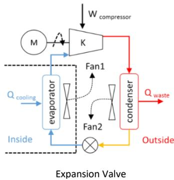
**Figure 1.** Air conditioning system used in current vehicles
