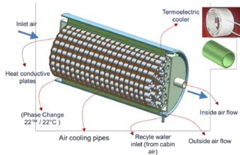
**Figure 9.** Newly developed cold storage system
