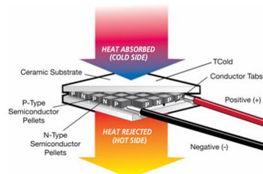
**Figure 4.** Thermoelectric cooler (Peltier heat pump) [8]
