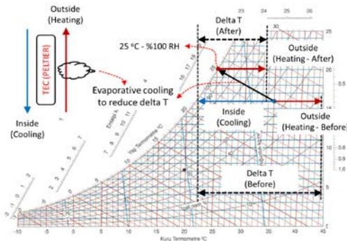
**Figure 6.** Existing situation and the new developed system on a psychrometric diagram
