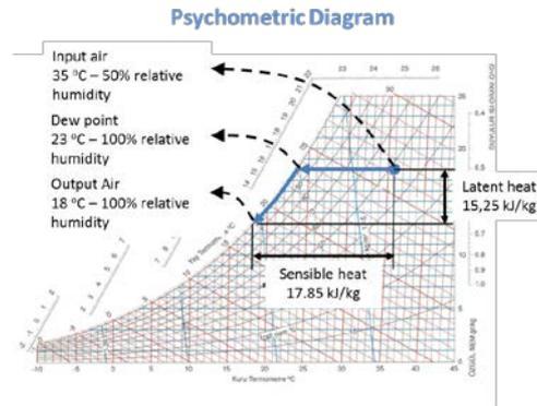
**Figure 3.** Current vehicle air conditioning system cooling group design (continued)
