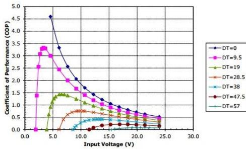
**Figure 5.** Thermoelectric cooler COP value/potential difference for different temperatures [9]
