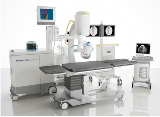
Figure 1. New generation electromagnetic Storz Medical Modulith SLK extracorporeal shock wave lithotripsy (ESWL) device
