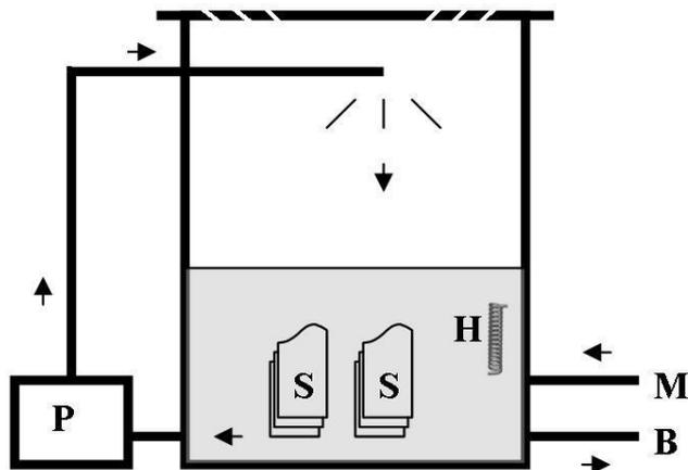
**Figure 1.** Schematic diagram of model recirculating water system, arrows indicate the flow direction. P: pump, S: surfaces, H: heater, M: make-up water inlet, B: blowdown outlet
