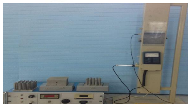
Figure 1 Experimental test setup including, 1. Power and control unit 2. Test area 3. Speedometer 4. Fan 5. Measuring and power cable 6. Air flow direction 7. Thermometers ( T_1 , T_2 , and T_3 ) 8. Manometer
