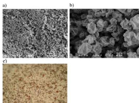
**Figure 2.** SEM images of DOX loaded SE microparticles. SEM images under a) 550X, b) 5000X c) light microscope image of SE particles (8 mg/ml PLGA) under 40X magnification.
