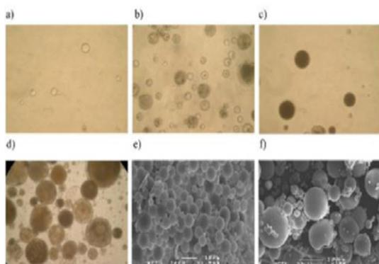
**Figure 1.** Morphology of DE microparticles. Light microscope images; a) 10 mg/ml PLGA, b) 30 mg/ml PLGA, c) 75 mg/ml PLGA, d) 100 mg/ml PLGA under 40X magnification. SEM images; e) 10 mg/ml PLGA, f) 75 mg/ml PLGA in the organic phase respectively.
