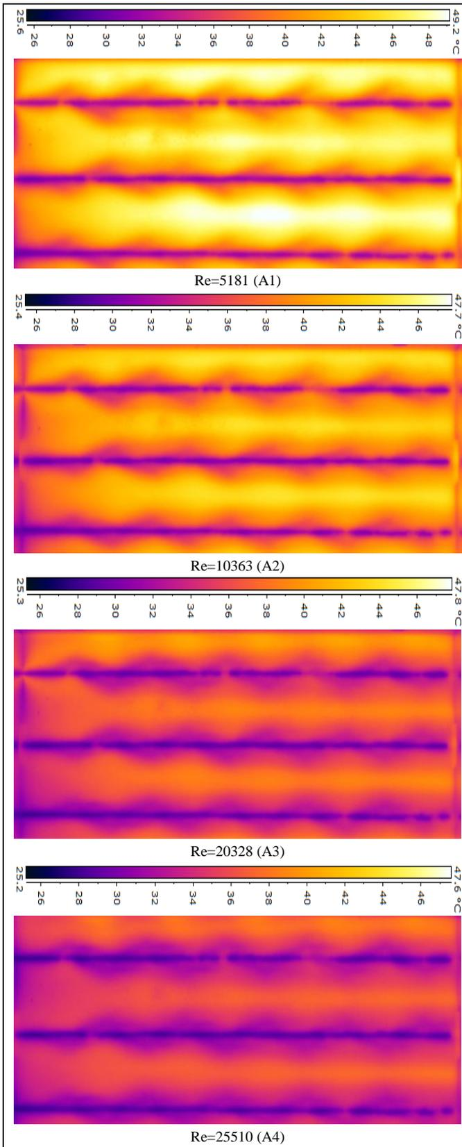
Figure 6 Temperature contours in the winglet channel obtained in different Reynolds numbers (A)
