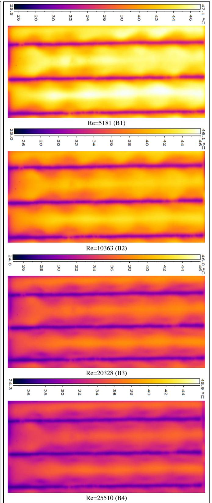
Figure 7 Temperature contours in the winglet channel obtained in different Reynolds numbers (B)
