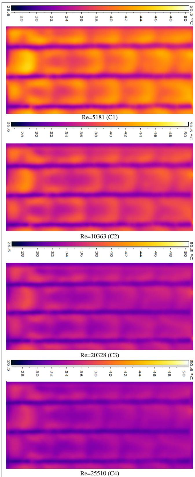
Figure 8 Temperature contours in the winglet channel obtained in different Reynolds numbers (C)
