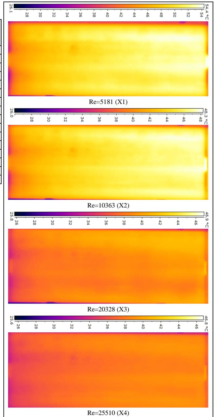
Figure 5 Temperature contours in the empty channel obtained in different Reynolds numbers
