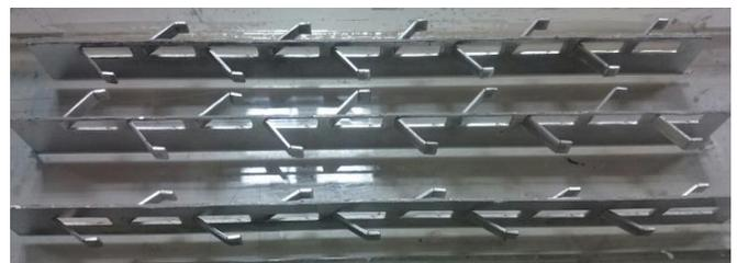
Figure 3 The winglet with 3 mm in height from the base and 30° angle.
