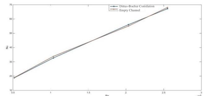
Figure 4 The validation of Nusselt number for empty channel
