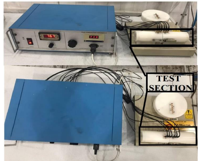
Figure 4 Heat conduction unit used in numerical calculations and experiments
